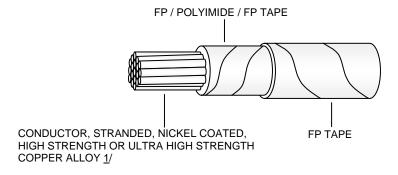
FP - FLUOROCARBON POLYMER, MODIFIED POLYTETRAFLUOROETHYLENE (PTFE)
